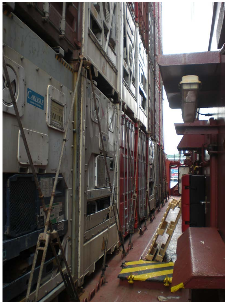
Photo 2: Stacks of containers lashed on the deck of a ship at the Hong Kong Kwai Tsing Container Terminals, 4 September 2008.
